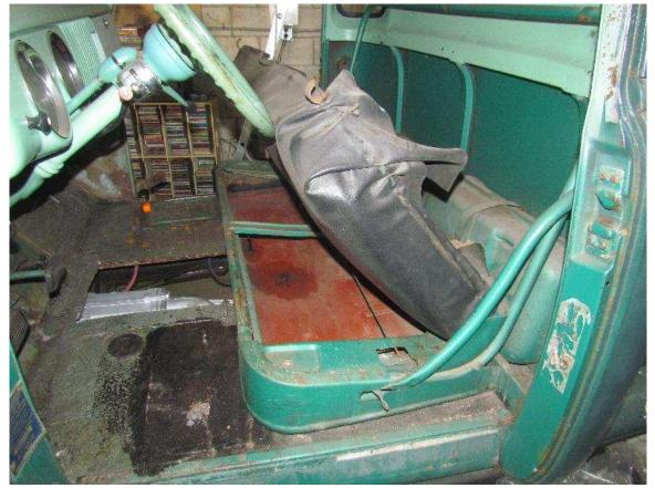
STEP 3..... Remove the two seat adjustment springs. The springs are located under the seat frame on the right and left sides. The springs are approximately 10 inches long. Be careful to note how the springs are attached to the seat platform and the seat frame..... so they can be re-attached properly when the frame is put back in the truck.
