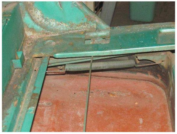
STEP 3A .. I don't know about the 47 2<sup>nd</sup> Series (Tom's truck) but the 55 1<sup>st</sup> Series (My truck) has sheet metal skirts on each side, held in with 5 sheet metal screws each. I remove the skirts at this point.
