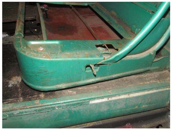
STEP 4..... Locate the four bolts holding the seat frame to the bottom platform. These bolts are located at each of the four corners of the seat platform. The bolts are stationary, and only the nuts are removed.
