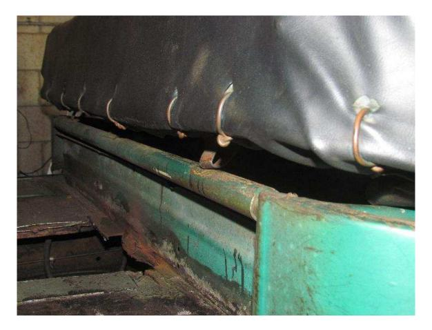
STEP 2..... Remove the back seat cushion. This is done by removing the screws on top of the three C-shaped tabs that loop over the top part (bar) of the seat frame. NOTE: These screws, if original, will be clutch-head screws. A special clutch-head screwdriver is needed to remove them. If the screws are to be discarded, a pair of vice-grips can be used to remove them.
